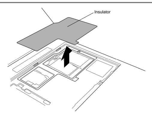
Figure 4-20 Removing the insulator
